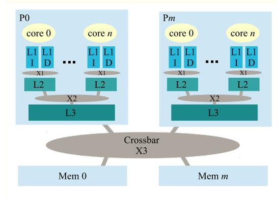
Figure 2: Multi-core system modeled using Sitar.
